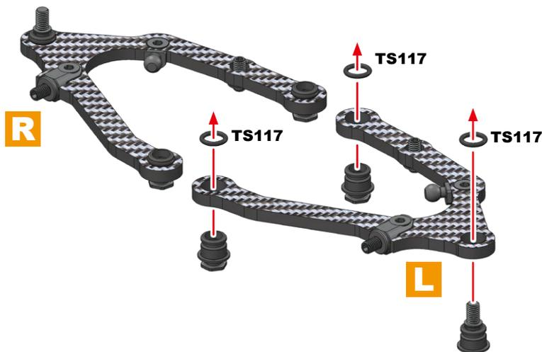
Ensure the O-Ring (TS117) is correctly seated into the groove on the sockets.
