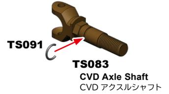
The C-clip (TS091) fits into the groove of the axle shaft. It can be easily fitted by hand without using tools such as pliers. Confirm that the C-clip rotates.
