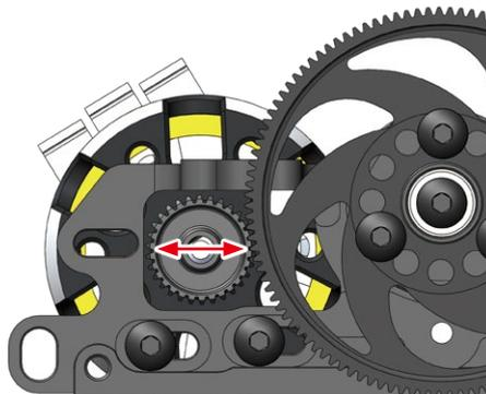
**Adjust the motor so the pinion meshes with the spur gear properly.**
