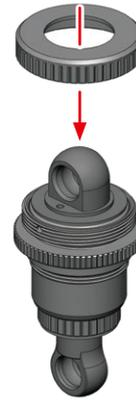
Gently place the shock top onto the shock membrane and allow the excess oil to drain under its own weight.
